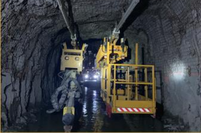
Two-way traffic via dual monorails
