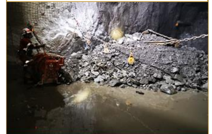
Mucking out a stope with a slusher
