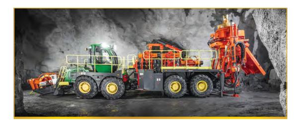
Torex's new Media Luna mine is being built with the future in mind and will utilize a hybrid fleet of vehicles and equipment. The mine's primary underground production fleet, underground mining support fleet and personnel transportation fleet will all be battery electric vehicles (BEVs). This will result in one of the largest BEV mining fleets in Latin America — and one of the largest in the mining industry more broadly.
