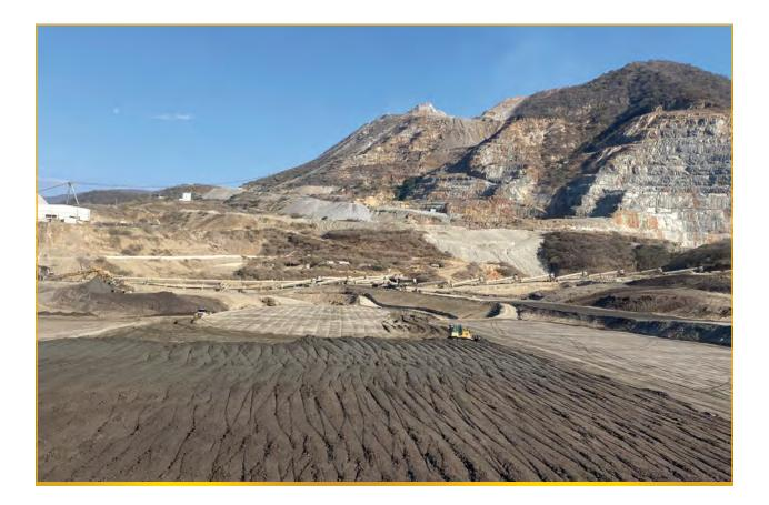
We filter our tailings through a filter press plant within our processing facility, which reduces the moisture content to approximately 17%. The remaining water is collected and sent back to the processing facilities for re-use. In 2022, approximately 1,241 megalitres (ML) of water was recycled through this process.
